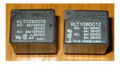
Test the new part(s) before installing them to make sure that the coil is operational (for a new relay the coil resistance should be approximately 400 ohms). With the new parts installed check all the relays before reassembly to ensure that the coil resistance for each band is approximately 200 ohms.
