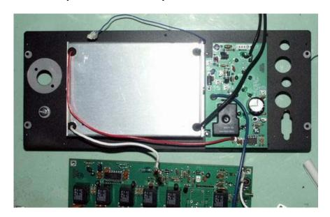
Rear panel with low-pass filter board attached
