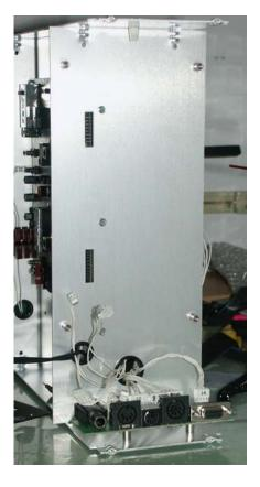
This figure is a rear view of the Jupiter on its left side with the back panel, DCIN board, Power Amplifier and low-pass filter board removed.
