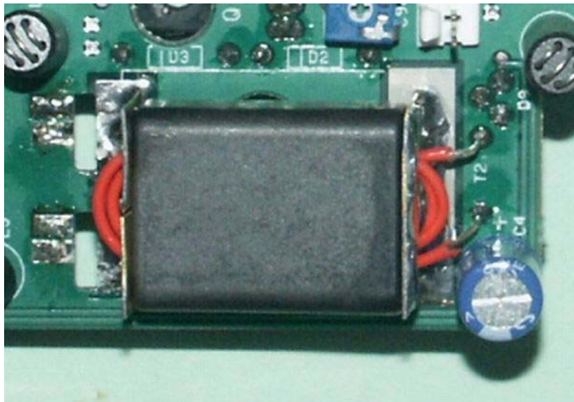
Figure 2: Enlargement of Transformer T2 with red wire primary (Note: Slots and solder pads to left end of T2)
