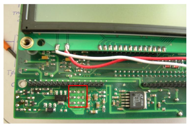
Picture illustrates removal of the 33 Ohm resistors only. Final change includes removing additional 47 Ohm resistor
