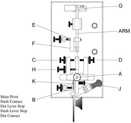
Dot Spring Damper Arm Dot Lever Tension Dash Lever Tension
