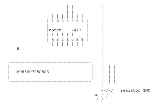
4) From the left vertical trace that was cut, solder a wire to pin 3 of the 7417 chip. It should look like this:
