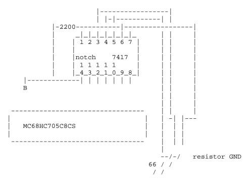
9) Pin 7 of the chip needs to have a wire soldered to it and run to ground. I found a ground on the right side of the resistor that is just to the right of the "66" label. Therefore, solder a wire that goes from
