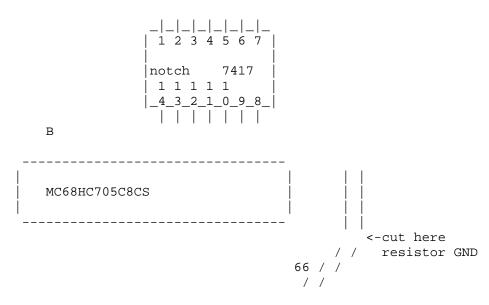
2) On the "66" side of the broken traces (diagonal part), you need to solder a jumper to connect these 2 traces together. It should look like this:
