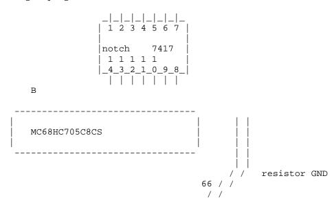
I have tried to show what this area looks like. Just to the right of the MC68HC chip are 2 vertical copper traces that come towards the front and then make a 45 degree turn towards the left. These traces go right through a connect to label marked "66".
