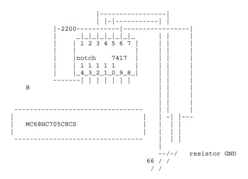
8) Solder another wire also to pin 14 of the chip and locate jumper B just to the left of the 7417 chip. Solder the other end of this wire to jumper B. It should now look like this:
